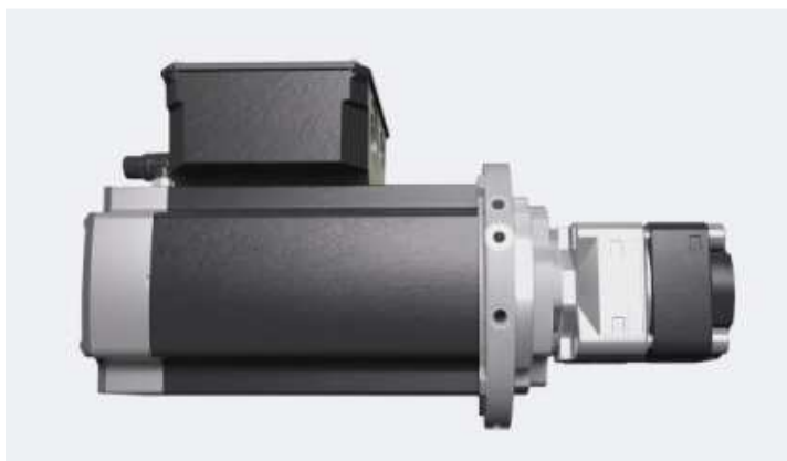
Fig. 2: In a nutshell: Coupling and pump support are not required with direct pump attachment, which also has the advantage of a shorter installation length and a smaller machine installation area, among other things | Image: Baumüller
